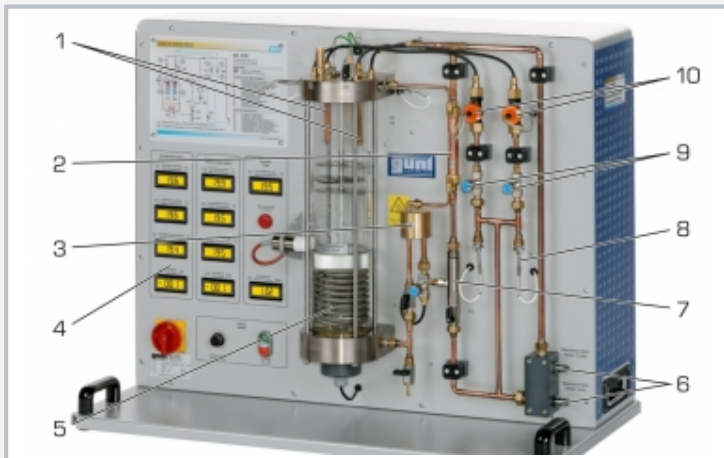
1 condensers, 2 heat exchanger, 3 steam trap, 4 displays for temperature, flow rate and pressure, 5 heater, 6 cooling water connections, 7 water jet pump, 8 temperature sensor, 9 valve for adjusting the cooling water, 10 cooling water flow rate sensor
