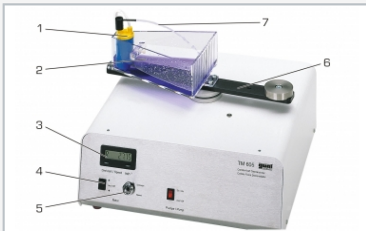
1 pump, 2 water tank, 3 speed display, 4 switch for direction of rotation, 5 speed adjustment, 6 rotating arm, 7 water jet
